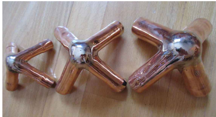
Variant of a pyramid tip connector The rule is: the sharper the better. This tip connector is not optimal.
